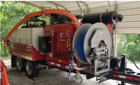
Ring-O-Matic 550VX High-CFM Hydro Vacuum Excavator and Trailer
