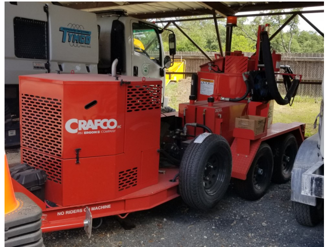
CRAFCO Super Shot 125 DC with 100 CFM Compressor (Crack Seal Machine)
