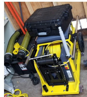
IBAK D059 Mainlite Portable System (pipeline and manhole inspection system)
