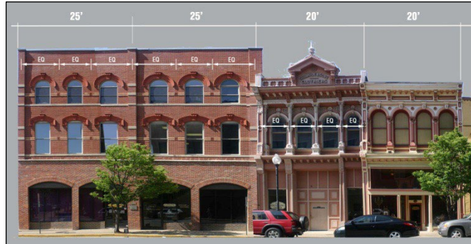
Figure 7-3 Illustration showing building articulation requirement
